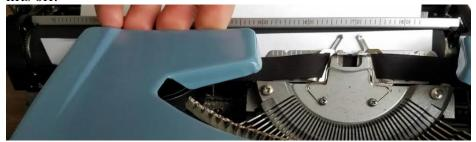
b. Shift the Spool Cam Lever left or right from its current position. The spools will now rotate in the opposite direction with each key strike.
