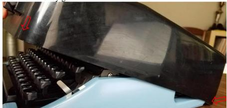
6. *If a typebar sticks*, lightly nudge the bar back towards its rest by applying pressure with a finger tip. Never attempt to bend a bar that is sticking—they snap very easily!!
