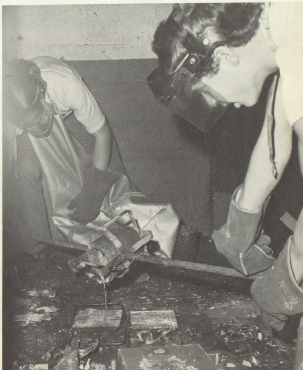
BELOW: Molten metal is poured into a casting in Metal Shop.
